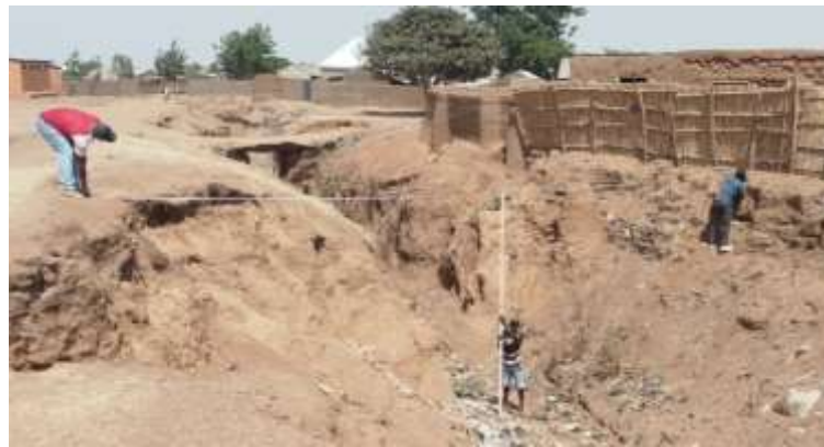
Plate II: Measurement of Gully Width and depth at Gombi 2
